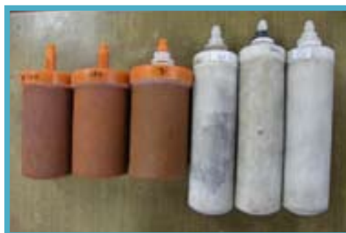
CSF candles researched at ENPHO Lab
