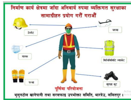
Display flex (Use of Personnel Protection Equipment for Workers at Construction Site)
